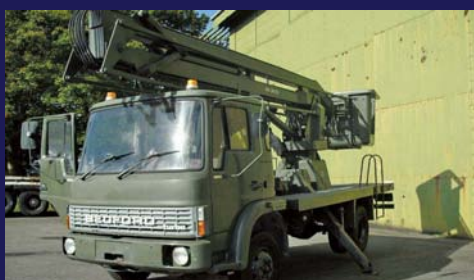
BEDFORD TL860 TURBO with Access platform Diesel Engine Bedford 330T Access platform with Spencer Lift 13.3Metre height capacity 340Kg swl, Hydraulic 2 Man Access (Cherry Picker) Stabilizer Legs Vehicle Length 7.80metres Width 2.45Metres Height 3.20Metres. Mileage 13,330 Hours 1735. £7,500
