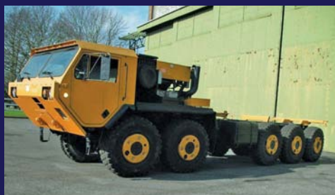
OSHKOSH 10X10 LHD Year 1989, 5 axle driving, 3 Axle Steering, Diesel Engine Detroit 8v92TA 500hp, Allison CLT755 Automatic Gearbox, Self Recovery Winch, 20ft Twist Locks, Michelin 16.00 R20 Tyres Vehicle Length 10.6 Metres Height 2.9 Metres Width 2.3 Metres Approx tare Weight 21tonnes Mileage 021025. Ex MOD Qty1 Guide Price £35,000
