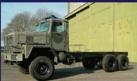
INTERNATIONAL 6X6 LHD PAY STAR 5000 , Chassis Cab, Diesel Engine Detroit 6V92T, Allison HT750 Automatic Gearbox, Vehicle Length 9 Metres Height 3.1 Metres Width 2.4 Metres Approx Tare Weight 8.5 Tonnes Mileage 27,855. Ex MOD Qty1 Guide Price £15,000
