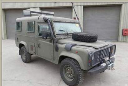
Land Rover 110 CAV 100 Enhanced Protected Vehicle , Land Rover Defender 110 is constructed of composite armour to defeat munitions up to B4 spec, 300 TDi Diesel Engine, R380 Gearbox, Upgraded Heavy Duty Front Vented Disc Brakes & Rear Disc Brakes, Salisbury Front and Rear Axles, Power Steering, etc. mileage from 58,000km, Excellent condition, Guide price from £25,000 (10 Available)
