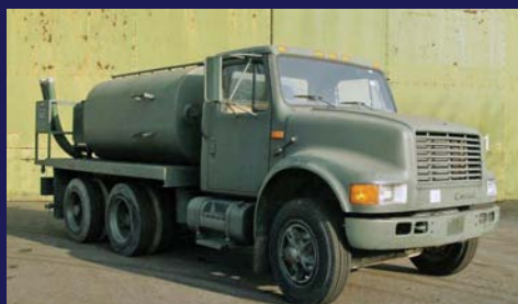
International 6x4 LHD Tanker , 1500 gallon tank Diesel Engine DT466, Allison HT653 Gearbox, Hale pump powered by John Deere 4cyl Diesel power pack. Vehicle Length 7.1 Metres Height 2.5 Metres Width 2.4 Metres Approx Tare Weight 8 Tonnes Mileage 2286 Ex Mod Qty1 Guide Price £10,000
