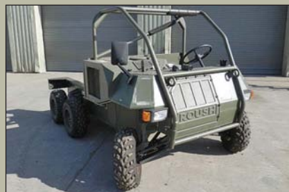
Roush 6x6 All terrain Load Carrier , Permanent 6 wheel Drive, Fully Automatic with Torque convertor, Aluminium Honeycomb construction for lightweight and strength, McPherson Strut front Suspension, etc. Mileage From: 130km, Hours from: 60hrs, Year 2006, Excellent condition, Guide price from £12,500 (6 Available)
