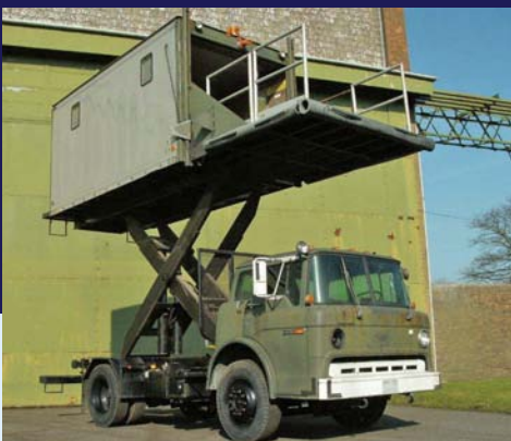
INTERNATIONAL 6X6 LHD PAY STAR 5000 , Chassis Cab, Diesel Engine Detroit 6V92T, Allison HT750 Automatic Gearbox, Vehicle Length 9 Metres Height 3.1 Metres Width 2.4 Metres Approx Tare Weight 8.5 Tonnes Mileage 27,855. Ex MOD Qty1 Guide Price £15,000
